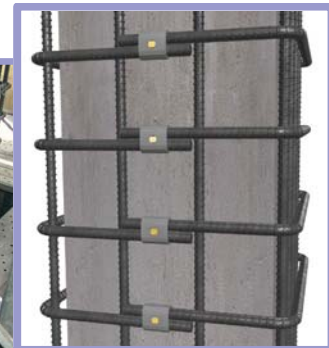
Reinforcements for SRC beam-Column joint
