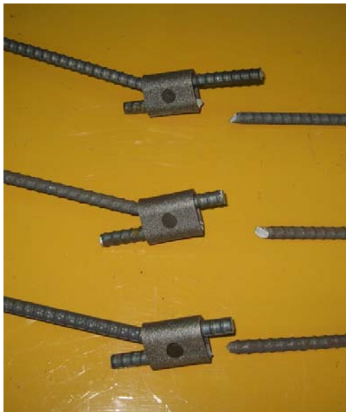
Specimens after tensile test
